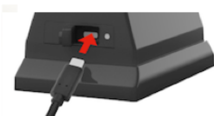
USB-C plug into the socket on the camera/ lithium battery
